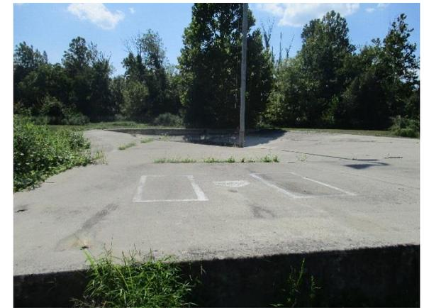
Parking spaces adjacent to the main building can be replaced with pervious pavement to capture and infiltrate stormwater runoff. A preliminary soil assessment suggests that the soils have suitable drainage characteristics for green infrastructure.
