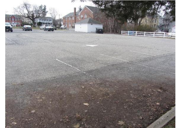
Parking spaces can be replaced with pervious pavement to infiltrate parking lot runoff. A preliminary soil assessment suggests that the soils have suitable drainage characteristics for green infrastructure.
